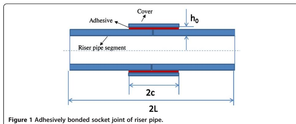
**Figure 1** Adhesively bonded socket joint of riser pipe.
