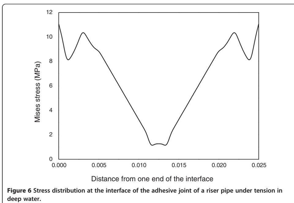
with the element sizes in this paper, which indicates that a singular stress field exists at the end of the interface.
