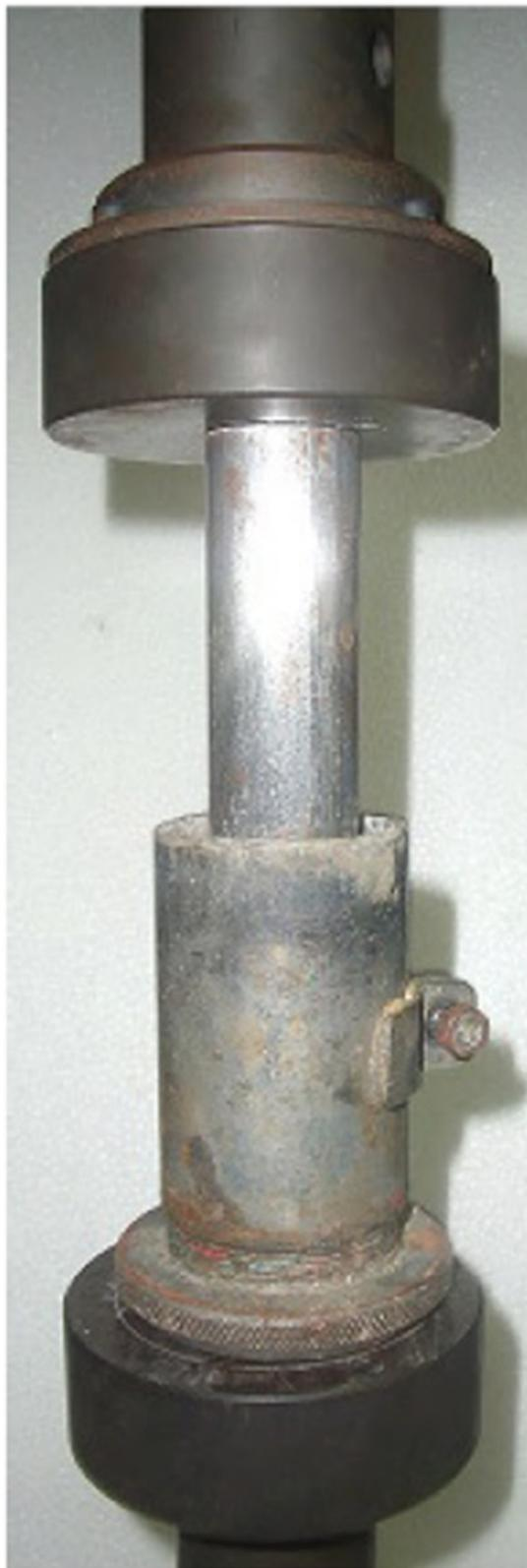
**Figure 2** Specimen during the static push-out test.
