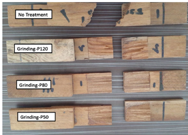
Fig. 8 Failure surface of wood adherend bonded joints
