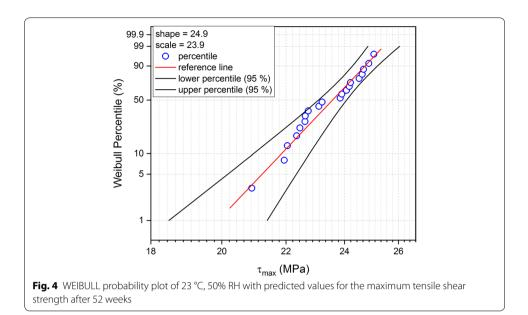
to specimens which show a comparatively low tensile shear strength. Based on these assumptions it is possible to include all experimental data to do a safety prediction for a certain condition considering a reliable variance.
