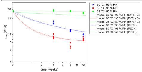
**Fig. 2** Maximum tensile shear strength  $\tau_{max}$  (dots) and combined functions to describe the temperature and humidity dependence of the maximum tensile shear strength referring to EYRING (solid line) and PECK (broken line)
