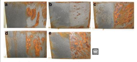
**Figure 8 Surfaces of coatings with and without sealant after salt-spray test.** Conditions: **a)** 1, **b)** 2, **c)** 3, **d)** 4 and **e)** 5. The left half area of each sample has sealed with epoxy.
