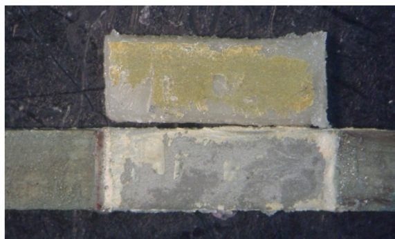
Figure 3 Optical microscopic images of a Co-Cr alloy with bonding agent application (G3) after flexural bond strength test, showing opaque layer remnants on metal surface (mixed failure).
