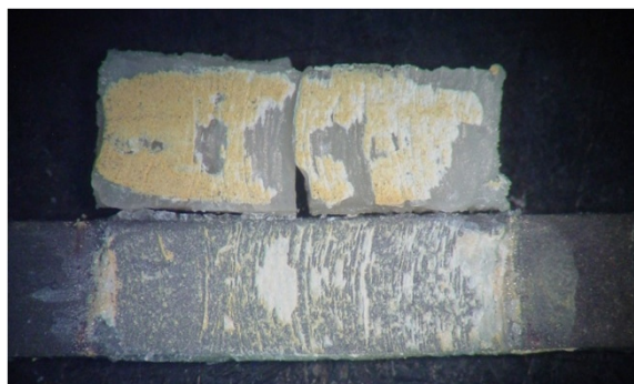
Figure 1 Optical microscopic images of a gold alloy with bonding agent application (G1) after a flexural bond strength test, showing opaque layer remnants on the gold surface (mixed failure).
