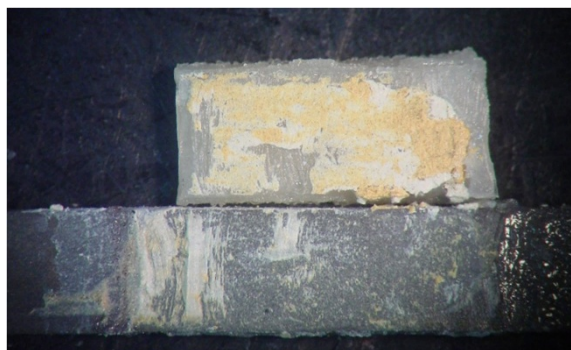
Figure 2 Optical microscopic images of a gold alloy without bonding agent application (G2) after flexural bond strength test, showing opaque layer remnants on the gold surface (mixed failure).
