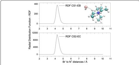
Figure 2 RDF for the distances between the Br<sup>-</sup> and ammonium<sup>+</sup> within the TEAB catalyst molecules for the both simulation systems CS1 and CS2. Upper: CS1-EB, the inset contains the illustration of the atom groups of the TEAB molecule for which the RDF was calculated. Bottom: CS2-EC.
