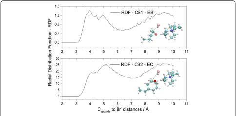
**Figure 3** RDF for the distances between the Br<sup>-</sup> of the TEAB catalyst molecules and one C atom of the epoxide molecules for both simulation systems. Upper: CS1. Bottom: CS2. The atoms among which the RDF is taken are illustrated in the inset sketch.
