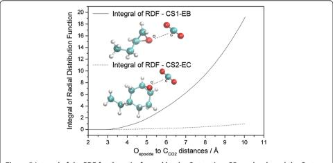
Figure 5 Integral of the RDF for the pairs formed by the C atom in a  $CO_2$  molecule and the O atom from the opened epoxide ring. Full line is the CS1. Dashed line is the CS2. The atoms considered in the pairs for which the integral of the RDF is taken are illustrated in the inset sketch.
