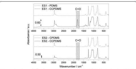
**Figure 1 Superimposed infrared spectra.** Upper: ES1 - reagent PDMS (dashed line) and product CCPDMS (solid line). Bottom: ES2 - reagent CPDMS (dashed line) and reaction mixture without indicating formation of a product CCPDMS (solid line).
