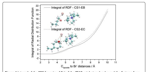
**Figure 4** Integral of the RDF for pairs of Br<sup>-</sup> of the TEAB catalyst molecules and the C atoms from the epoxide molecules for both simulation systems. Full line is the CS1. Dashed line is the CS2. The atoms considered in the pairs for which the integral of the RDF is taken are illustrated in the inset sketch.
