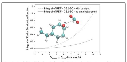
Figure 6 Integral of the RDF for the pairs formed by the C atom in a  $CO_2$  molecule and the O atom from the opened epoxide ring for system CS2-EC with and without considering catalyst. Dashed line is the original CS2-EC with catalyst. Full line is the CS2-EC without the presence of catalyst molecules. The atoms considered in the pairs for which the integral of the RDF is taken are illustrated in the inset sketch.
