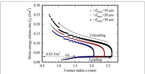
**Fig. 5** Strain energy release rate  $G_Z$  as a function of the contact radius a. An approximately constant value of  $G_Z$  at the end of each step is observed in the loading process; on the contrary, in the unloading process,  $G_Z$  varies with the receding of a. The approximated value of 0.03 J/m<sup>2</sup> at the end of each step in the loading process is estimated to the work of adhesion  $\Delta y$ . The initial contact of the first step is shown as a
