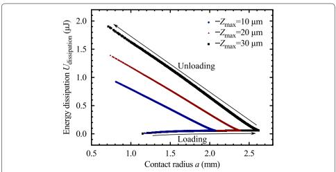
**Fig. 6** Total energy dissipation  $U_{\text{dissipation}}$  as a function of contact radius a. Linearity between  $U_{\text{dissipation}}$  and a is observed in the unloading process (receding contact)
