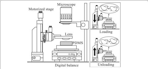
**Fig. 2** Schematic illustration of the measurement system (*left*) and loading–unloading processes (*right*). The gross displacement was controlled by the motorized stage, and the force and contact area were measured by using the digital balance and microscope
