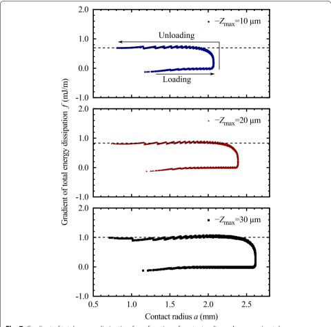
**Fig. 7** Gradient of total energy dissipation f as a function of contact radius a. An approximately constant value of the gradient f is obtained in the unloading process (receding contact): f = 0.71 mJ/m ( $-Z_{\rm max} = 10 \ \mu {\rm m}$ ), f = 0.83 mJ/m ( $-Z_{\rm max} = 20 \ \mu {\rm m}$ ), f = 1.03 mJ/m ( $-Z_{\rm max} = 30 \ \mu {\rm m}$ )
