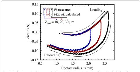
**Fig. 4** The loading–unloading curve of  $-Z_{\rm max}=10$ , 20, 30 μm. The measured force F and calculated force F(Z,a) are plotted as a function of the measured contact radius a. The calculated forces is calculated by substituting the measurements of Z and a into F(Z,a) of Eq. (6); R=0.2076 m, k=10.5 kN/m, and  $E^*=2.67$  MPa with an RMSE between F(Z,a) and F was 0.6 mN
