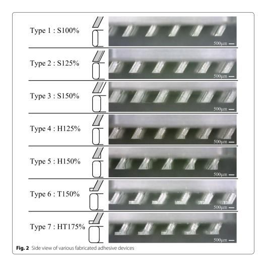
elongation) and the width 1.5 times larger than Type 1 (denoted as T150%). Type 7 has tips elongated 1.25 times at the rear and 1.5 times at the front (i.e., 75% wider) compared with Type 1, (denoted as HT175%).
