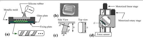
**Fig. 1** a Schematics of the device fabrication process, **b** a picture of fabricated device, **c** a schematic of *side* and *top views* of each tilted beam structure, and **d** schematics of experimental setup for measuring device adhesion versus pulling angle
