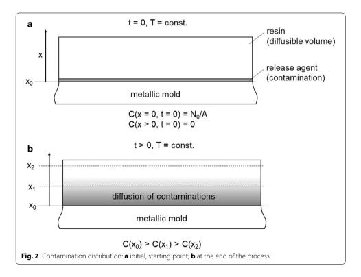
resin with release agent molecules decreases with increasing x ( $C(x_0) > C(x_1) > C(x_2)$  for  $x_0 < x_1 < x_2$ ).
