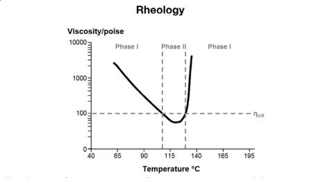
**Fig. 3** Correlation of viscosity and temperature for a representative prepreg-system [23] with the schematically representation of critical viscosity and the relevant phases
