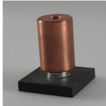
Fig. 2 The stamp-to-plate specimen used in the centrifuge tests: (left) metallic stamp bonded to the CFRP adherend; (right) specimen with copper mass body
