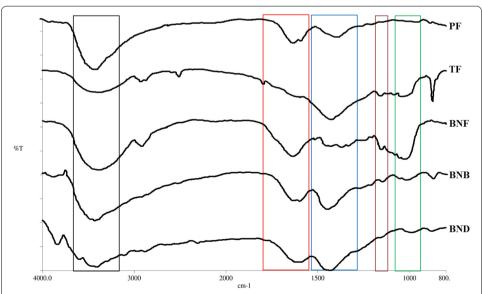
**Fig. 5** FTIR spectra of cured glue mixtures with additional BN bark filler: *PF* phenol formaldehyde, *TF* technical filler, *BNF* benuang bark filler, *BNB* glue mixture with 10 PF: 1.5 TF: 0.5 BNF, *BND* glue mixture with 10 PF: 1 TF: 1 BNF
