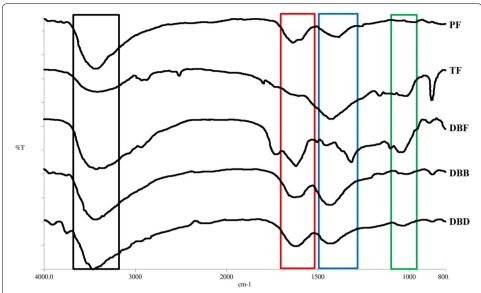
**Fig. 6** FTIR spectra of cured glue mixtures with additional DB bark filler: PF = phenol formaldehyde, *TF* technical filler, *DBF* duabanga bark filler, *DBB* glue mixture with 10 PF: 1.5 TF: 0.5 DBF, *DBD* glue mixture with 10 PF: 1 TF: 1 DBF
