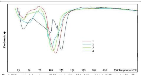
**Fig. 4** DSC analysis of glue mixtures: (1) PF: technical filler: DB bark filler = 10: 1: 1, (2) PF: technical filler: BN bark filler = 10: 1: 1, (3) PF: technical filler: bark filler = 10: 2: 0, and (4) PF: technical filler: bark filler = 10: 0: 0
