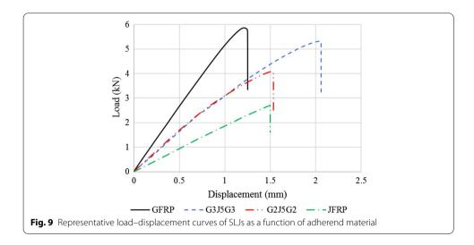
Similar to the failure load, the rigidity of the joints also varied as a function of the adherend material, going from highest for the GFRP joints to lowest for the JFRP joints. The pure jute joint (JFRP), presented the lowest joint rigidity and a completely brittle behaviour. The lower ductility of the jute composite does not accommodate the overlap edge rotation due to load-axis eccentricity, therefore, it fails catastrophically earlier in the displacement.
