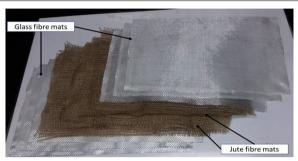
**Fig. 1** Natural and synthetic fabrics used and stacking sequence for the fabrication of the hybrid composite adherends 3-layer glass fibre hybrid composite case  $(G_3J_5G_3)$
