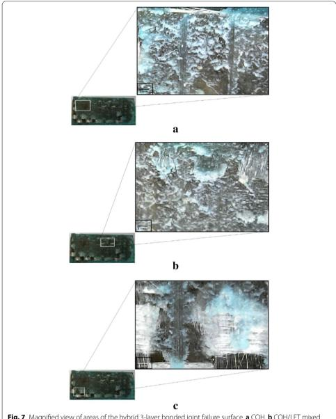
**Fig. 7** Magnified view of areas of the hybrid 3-layer bonded joint failure surface, **a** COH, **b** COH/LFT mixed mode and **c** TLC/LFT mixed mode
