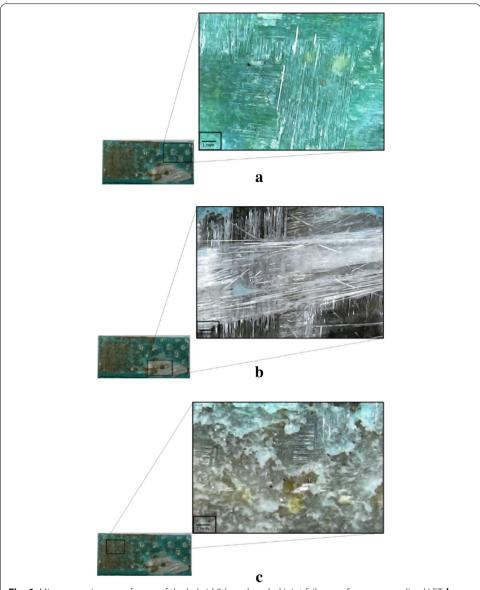
**Fig. 6** Microscope images of areas of the hybrid 2-layer bonded joint failure surface, **a** generalized LFT, **b** generalized delamination and  $\mathbf{c}$  TLC/LFT mixed mode
